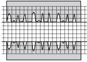
Graphs showing a cylinder liner before honing (left) and after honing by a Flex-Hone (right), which results in a super-smooth finish
